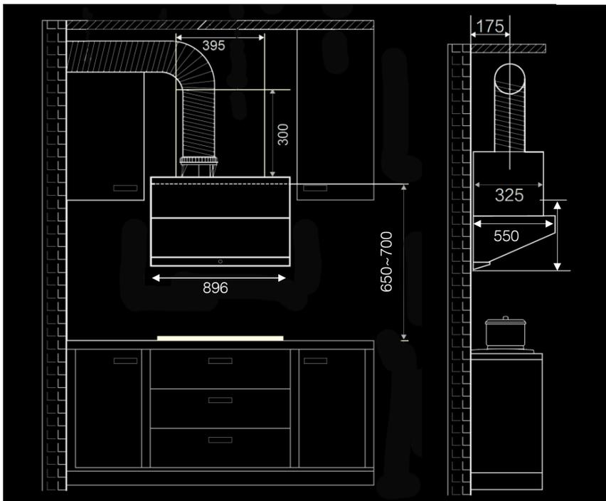
Note: This installation height is only applicable for kitchens with electric stove, if installed above a gas stove, the installation height should be in accordance with the installation height requirements of gas stove.
