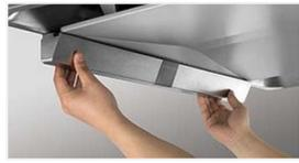
The **Oil Collector** in TISCA 90 has a capacity of 1.5 L needing occasional cleaning. Heavy oil and grease from the fumes hit the oil net and get accumulated in the collector while the lighter smoke is thrown out through the duct.
