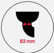
**MagnaFeed Inlet:** The MagnaFeed Inlet of the Magnus Cold Pressed Juicer is 83 mm in diameter which helps it take in whole fruits like a big apple, pear, oranges, etc. without the hassle of cutting them.
