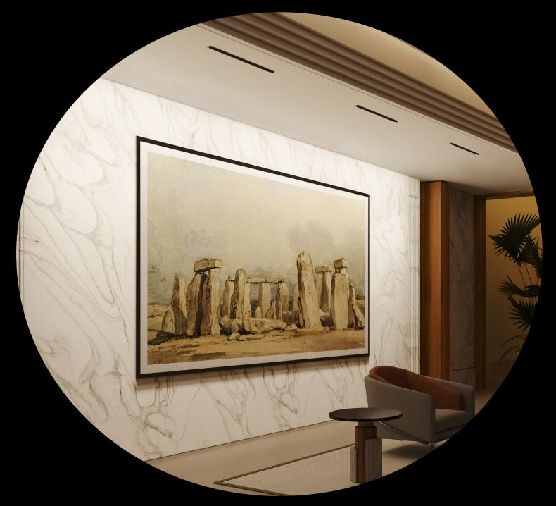
Wall washing is a special and unique effect that illuminates a vertical surface with flawless and even brightness. It is the element that draws attention to your textured wall, wall display, entrance or fireplace and makes it noticeable. The light fittings that deliver such effects not only need to produce a high quality light output but also need to be technically efficient.
