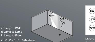
The distances from lamp to wall, lamp to lamp and lamp to floor should be in the ratio of 1:1:3 (meters). For example, if the lamp is installed at a height of 3 meters above the floor, then the distance of the lamp from the wall which the lamp is illuminating should be 1 meter and its distance from adjacent lamp should be 1 meter.
